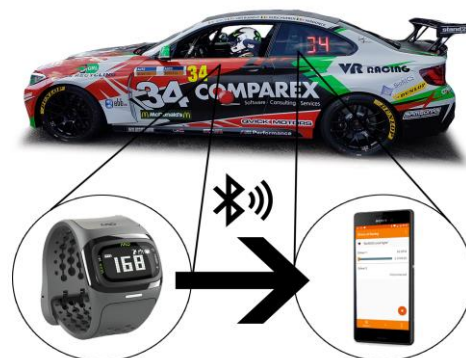
Figure 1. Schematic overview of the stress level monitoring system in a race car
